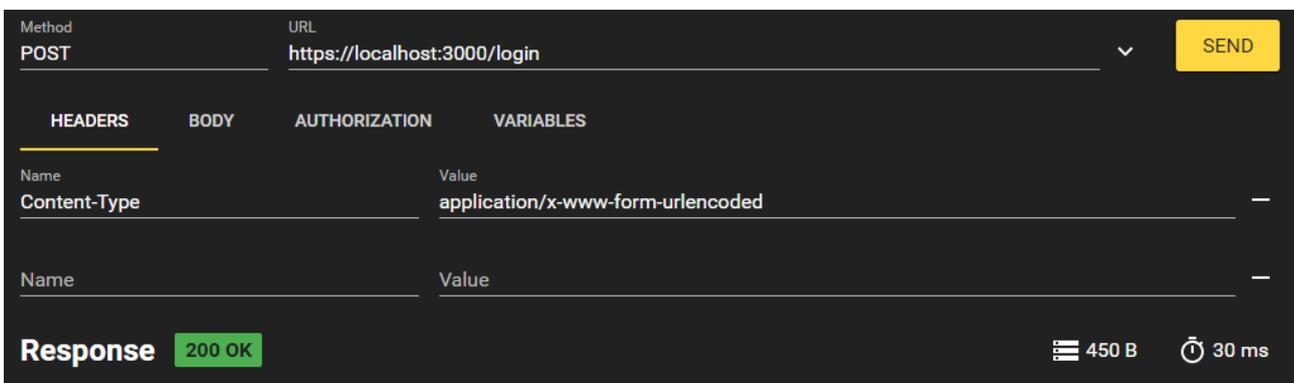
The screenshot shows the Postman interface for a POST request to `https://localhost:3000/login`. The 'HEADERS' tab is selected, showing a single header: `Content-Type: application/x-www-form-urlencoded`. The 'Response' section at the bottom indicates a `200 OK` status with a response size of `450 B` and a response time of `30 ms`.
